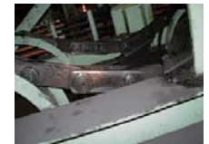
Dummy Bar Car Chain inside a dummy bar car
