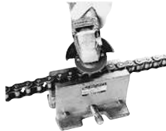
Fig. 2 Grinding the pin ends
