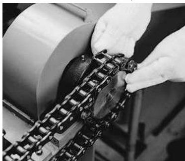
Fig. 8 Connecting on a sprocket
