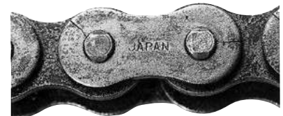
Fig. 32 Hydrogen embrittlement cracking
