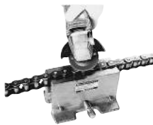
Figure 3: Grinding Down Pin Ends
