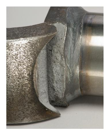
Our welds are tested for proper weld penetration, to ensure that each weld has achieved optimum strength and each link will provide maximum durability.
