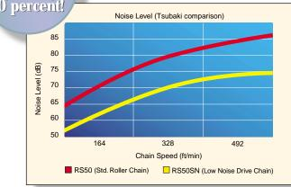
Comparison of Low Noise Drive Chain to Prelubricated ANSI Roller Chain.
